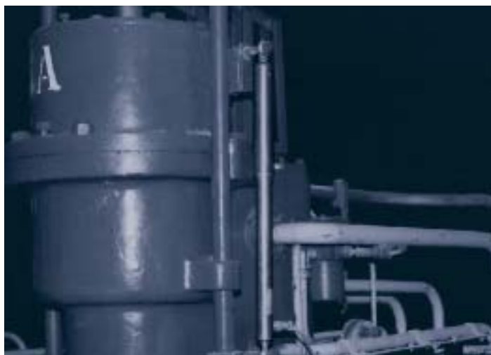
Heavy industrial LVDT monitoring valve position
